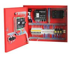
Deepsea 6120 is an auto mains failure controller for single generator, it can monitor and protect the generator working all the time. it has a LCD display which clearly shows the status of the engine. this controller include seven inputs and six outputs. This controller can also be programmed using the frong panel or by using DSE configuration Suite PC software.
