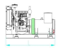
Open Type (Standard Configuration) Overall Size: 3000×1270 ×2040mm(L\*W\*H)
