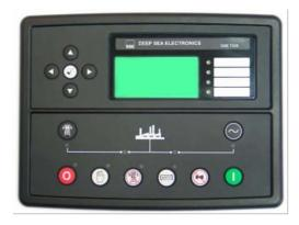
The DSE7320 is made by DEEPSEA in England and is a new control module for single gen-set applications, and it is an Automatic Start Control Module and is simple to operate, and the module includes USB,RS232 and RS485 for expansion device connectivity.
